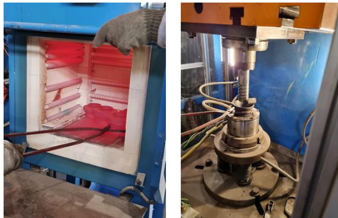
Figure 3: Experimental setup at ITUN (left-hand side: muffle furnace for pre-heating; right-hand side: hydraulic piston press)
